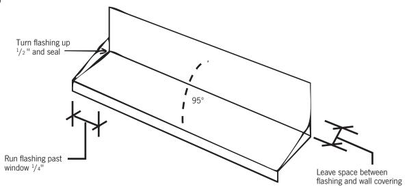
Recommended method for flashing a window or door head or at any ledger that stops in the middle of a wall. Turn up flashing to form "endcaps" and seal making sure that the length of the flashing overhangs the protrusion by 1/4" on each side. The wall covering is left up off the bottom bend of the flashing to help keep the 5° slope.
